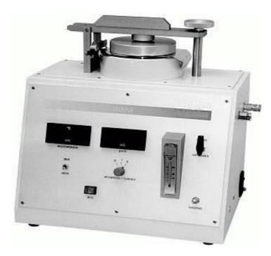
The inserted sample divides the permeation cell into an upper and a lower part. In the upper part of the permeation cell, a constant water vapor pressure (relative humidity) is set using saturated sulfuric acid solutions, a constant water vapor pressure (relative humidity) is set in the upper part of the permeation cell. The
