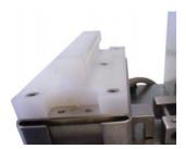
To determine the ink abrasion resistance and dirtiness characteristics on different supports (paper, cardboard, ceramic, etc.)
