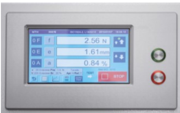
Display of the tensile tester with two separate buttons for Start and Stop.
